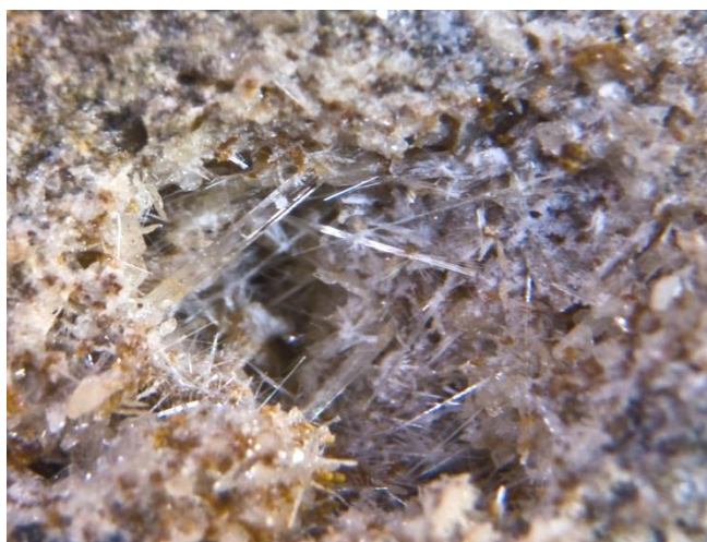
Figure 1. Micrognacious structure of wollastonite (magnified 1700 times).
