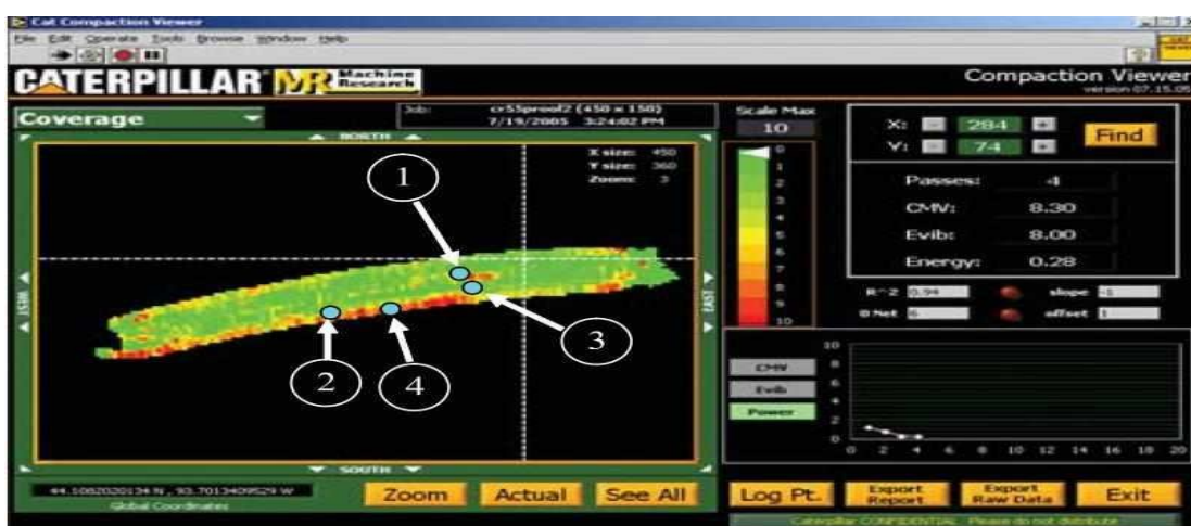
View of the state of the layer density on the monitor of the integrated density system.
