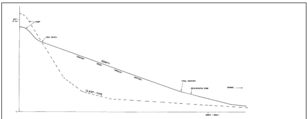
Fig. 1 Typical profiles of Dowty and clasp-type retarder yards
