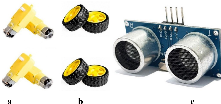
Figure 4. a) DC Motor b) Wheels c) Ultrasonic Sensor
