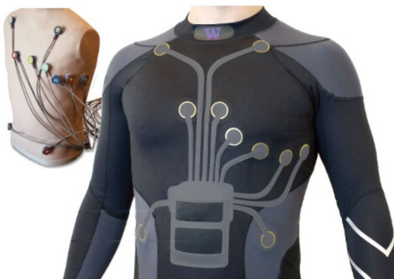
Figure 2. The use of sensor-based clothing in smart textiles to detect human body health indicators.
