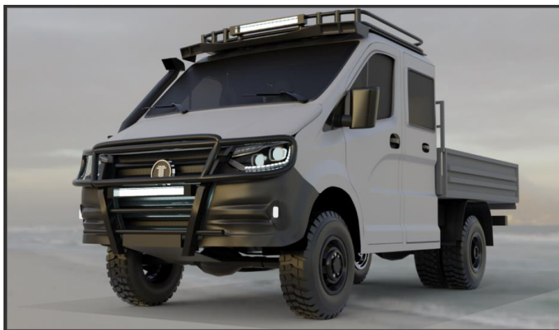
Fig. 5. A compact truck (based on Gazelle NN) designed in Blender with additional luggage racks for protection and cargo
