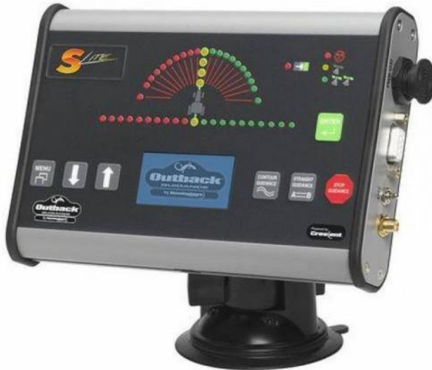
Figure 2. The base unit of the Outback S-Lite parallel driving system.
