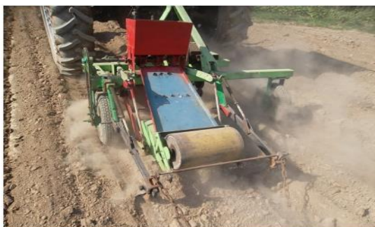
Figure 2. A combined unit with a star-shaped chain drive in the transmission mechanism
