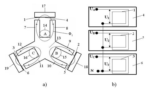
a - a magnetic core of a three-beam star-shaped rod
